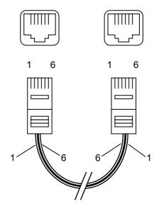
Figure 1: Modular cable, cross wired
