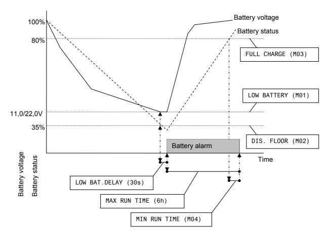
Figure 10: battery alarm settings
