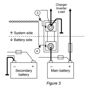
12. Make a connection between the minus of the secondary (starter) battery and the system side (figure 3) of the shunt.
