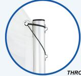
THROAT, Attach lacing lines with reef knots.
