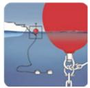
Only the lower swivel shall be used for mooring. Do not expose the buoy to a load of more than 60% of its total buoyancy. All mooring shall be checked for wear and tear twice a year.
