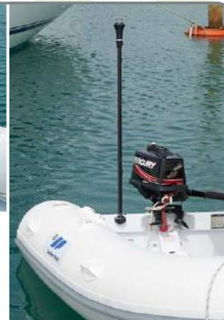
The i360 meets the required standards for an all-round white navigation light for power and sailboats under 12 metres, and kayaks & canoes. To maximise battery life we have used a high quality, Japanese made, Nichia power LED and a high efficiency digital circuit. It is lightweight, and IP67 rated for dust and water ingress. AA batteries mean many more light hours for your dollars when compared to AAA, and as it's battery powered there's no need for external wiring and switching.
