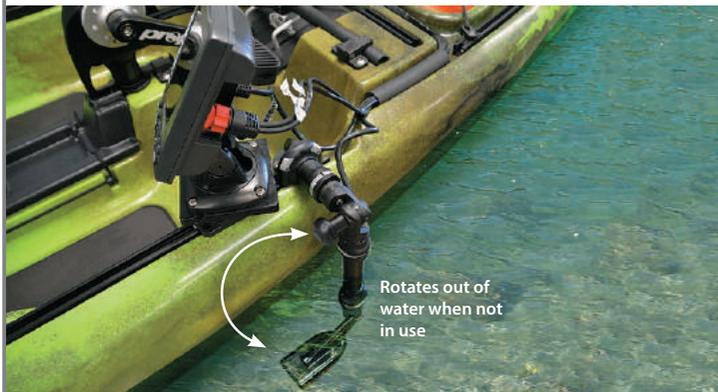
Rotates out of water when not in use
