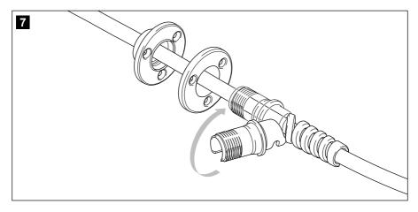
With the bulkhead fittings on the hose, wrap the split grommet (figure **B**, item 3) onto each hose, between the bulkhead fitting and mounting plate, oriented as shown.
