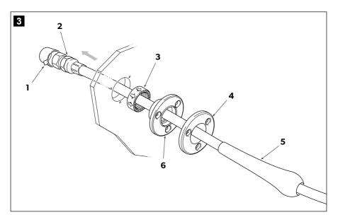
With the dust caps still installed, feed the hoses from the outside of the boat through the newly drilled holes, inside along the gunwale or rigging tube to the desired steering system component. The mounting plates, knurled nuts and bend restrictors must remain outside the boat hull.
