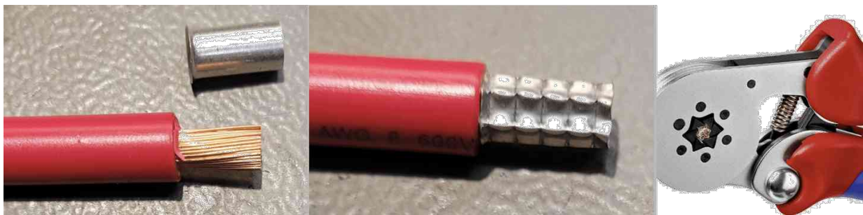
Hexagonally crimped bootlace ferrule
