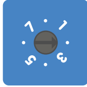
Rotary switch set to position 2
